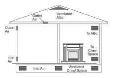
Figure 5 - Ventilation Air from Outdoors
